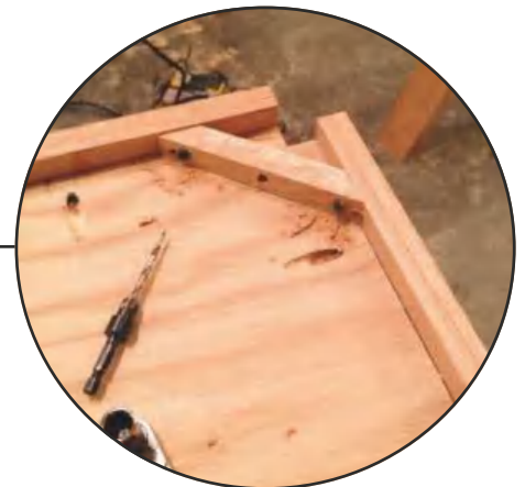
STEP 5. You can now add braces for the hex bolts to support the corners. These require a counter-sunk hole for a corner screw
